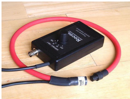
Figure 28. An example of the Rogowski coil current sensor—model 8000 of Rocoil [68].
