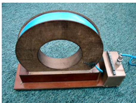
Figure 35. The air-coil sensor designed for investigations of magnetic pollution.
