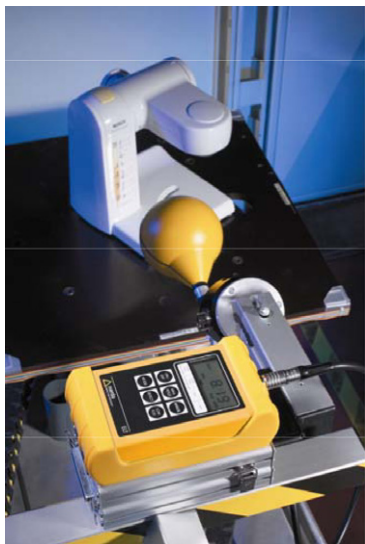
Figure 34. An example of a search coil magnetometer used for testing electromagnetic compatibility (with permission of Narda Company).
