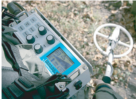
Figure 40. An induction search coil as a tool for the detection of metal objects (with permission of DCG Detector Center).
