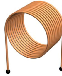
Figure 1. The simplest coil-based sensor for flux density and magnetic fields.
